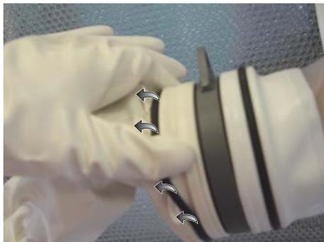
4. Roll the outer edge of the glove from the inner groove of the glove port into the glove-sided outer groove.
