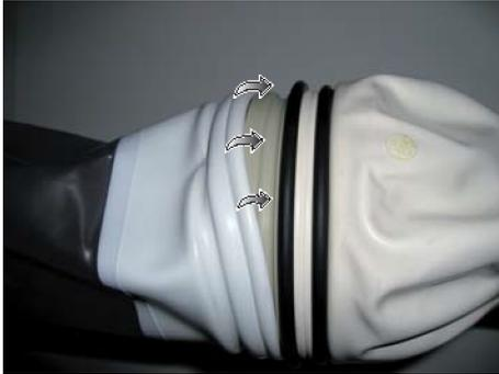
3. Roll the O-ring of the sleeve from the glove ring back on to the sleeve.
