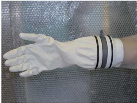
3. Roll the O-ring of the glove from the glove port onto the glove.
