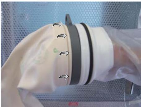
8. Remove the glove to be exchanged by pulling it from the glove port through the sleeve to the outside.
