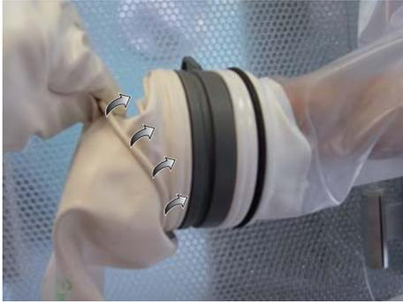
7. Roll the outer ring of the glove to the inner, glove-sided groove of the glove port.
