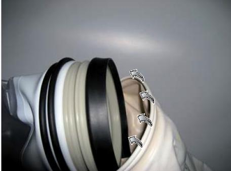
2. Roll the O-ring of the glove from the glove port back onto the sleeve.
