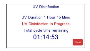
If the safety screen is removed or the "cancel" button is pressed the cycle will terminate. At the end of the cycle (or if aborted), the following screen is displayed. Follow the instructions to return to normal operations or return to UV setup.
