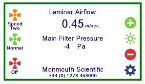
SPEED 2 is a preset that can be set higher or lower then NORMAL. An example of it's use could be to set higher to rapidly purge the cabinet<sup>\*\*</sup> or lower to conserve energy when a non-critical task takes place within the cabinet.
