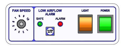
The booth is started by first operating the green rocker switch on the control panel. The Red airflow monitor warning light will flash until the correct airflow is achieved.
