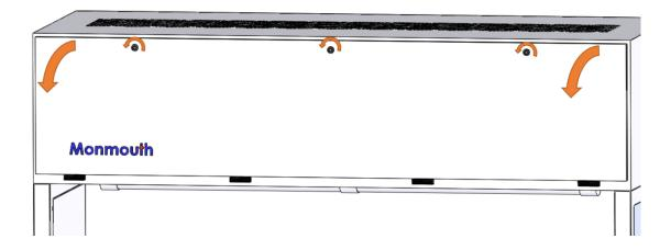
Working inside the enclosure, slacken the 4 off clamp knobs clamping each fan box module to the filter. Work each side in turn to raise the fan box evenly, until a sufficient gap is present to enable the removal of the HEPA filter which should freely slide out of place.
