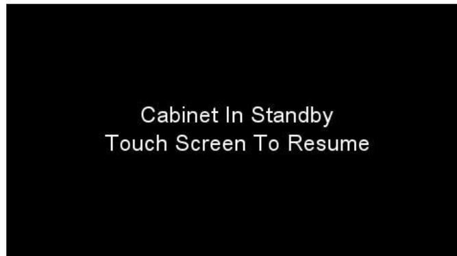
Touching the screen will wake the cabinet , open the sash, start the fans and resume operation.
