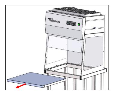
• Check for alignment and fix the cabinet enclosure to the base stand (2 screws per side).
