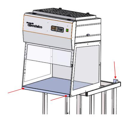
• Working underneath the tray, undo the tray fixing screws (3 per side) and rear nuts (2 off) and slide the tray forward to remove.
