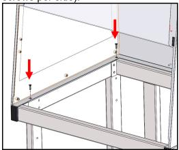
• Slide the tray back into position and refit the tray fixing screws (3 per side) and rear nuts (2 off).
