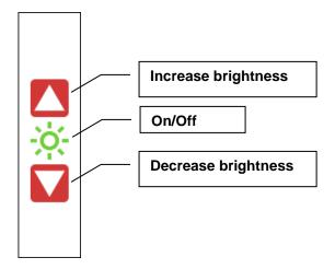
By pressing the "Up" or "Down" arrows you can adjust the brightness. Pressing the "Lighting" icon will turn the light off. Pressing the icon again will turn the light on.
