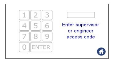
Press "0127" then "Enter" to start the cabinet. The screen will automatically open the sash to its normal working position, the fans will start and the lighting will illuminate.
