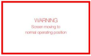
In addition, there is an integrated safety system that automatically prevents the sash from closing should an obstruction be detected. If an obstruction is detected the the sash will stop moving and retract upwards a short distance. A warning is displayed in the event of activation:
