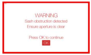
Remove the obstruction and press "OK". This will reset the system and the sash will attempt to close.
