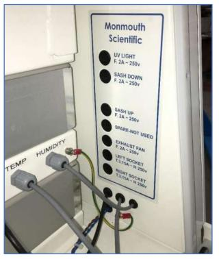
• Use a suitable flat head screwdriver to open the fuse holder. Replace fuses with type T, 5 x 20mm. Use Amp rating shown on label to select correct fuse.
