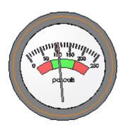
When the reading is within the green segment, this indicates that airflow through the cabinet is within the required parameters.
